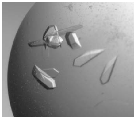
Figure 1 Photomicrograph of crystals of AVP. Prism-shaped crystals of AVP obtained by microseeding were used for X-ray diffraction. The typical crystal dimensions were 0.05 \times 0.15 \times 0.50 mm.
